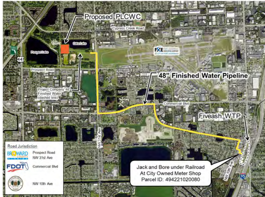
Figure 2-8: Finished Water Pipeline from PLCWC to Fiveash
